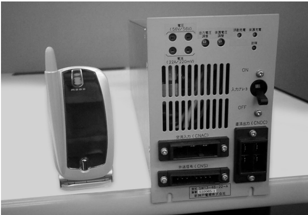
図9 直流電源装置の外観 Fig.9 Appearance of DC Power System.
