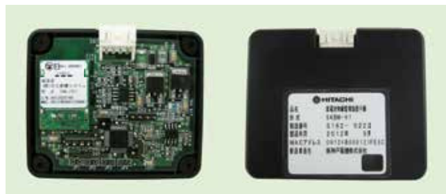
図3 無線子機基板 Fig.3 Appearance of wireless device
